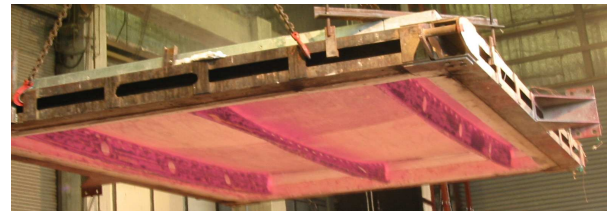
Deformed shape after the fire test shows joists glowing and the buckled shape of the mid joist as it was lifted up some 10 minutes after the furnace was shut down.
