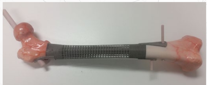
3D printed implant Titanium for patients with bone cancers.
